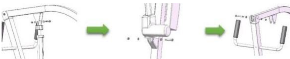
Fig. 3. Installation of lift arm
