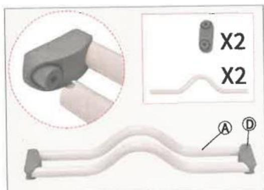
2. Insert the front bar(A) to the connector piece(D) along with its slots.
