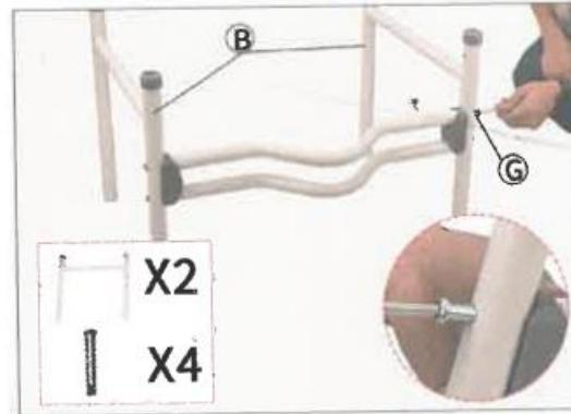
3. Insert the installed part(step 2) to the side racks(B) and insert the screw bolts (G) to the corresponding holes, fixed it with the Allen key(G).
