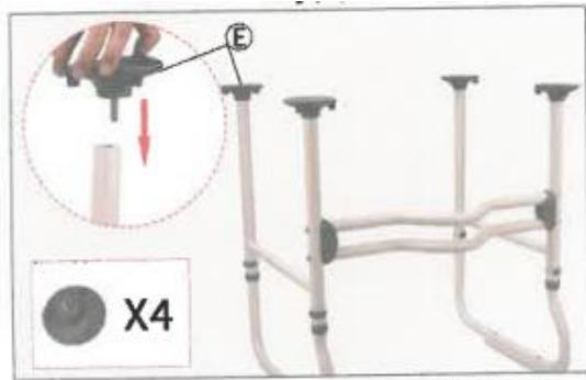
6.Twist to fix the suction foot pad(E) to the corresponding part in the installed frame (step 5).
